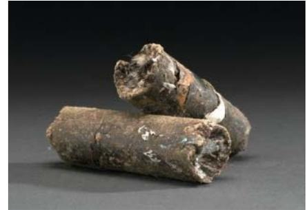
**Photo 1: Typical Refuse Derived Fuel (RDFuel) Pellet**
