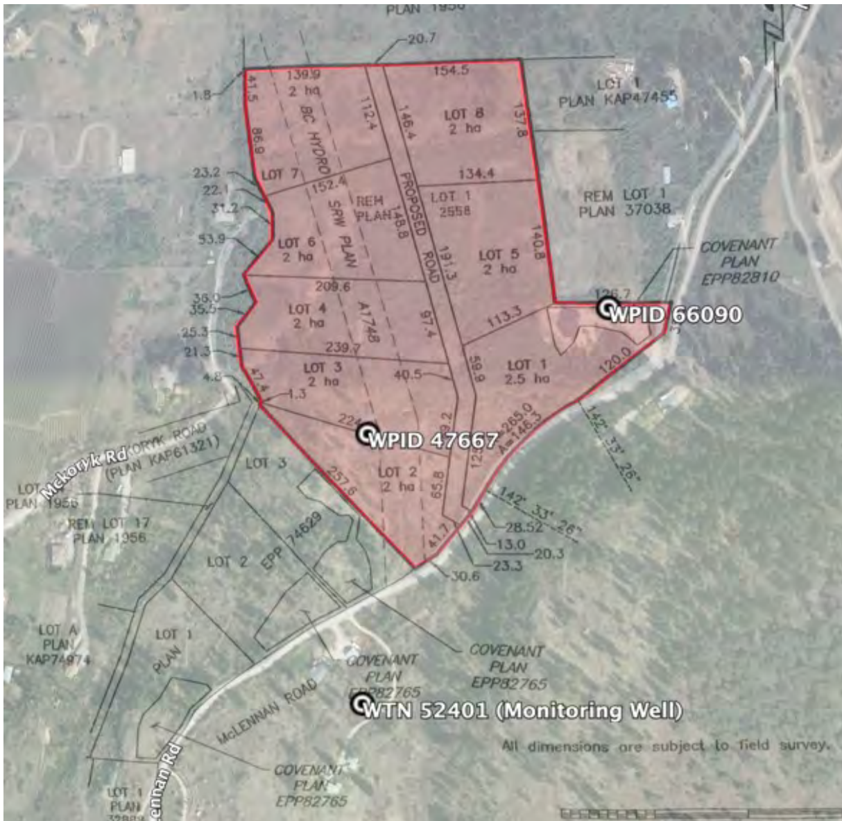
Figure 2: Image showing the site boundaries, proposed lot lines and location of existing wells onsite and the off-site monitoring well.
