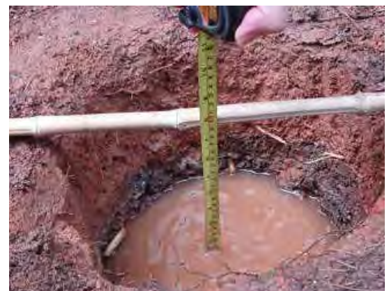
Image 3: Soil Drainage Rate- Percolation test
