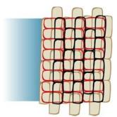
Every second course of sandbags should be set back a quarter (1/4) of a sandbag width, both on the river side and the land side of the dike, producing step-like appearance.
