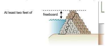
Sandbag dikes will compact when they get wet, which can reduce the available freeboard. The amount of compaction due to wetting increases with the size of the dike. Add at least five per cent to the required height of the dike to account for compaction. For example, add three to four inches for a six foot dike to account for compaction due to wetting.
