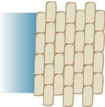
Rotate bags 90 degrees when laying second course of sandbags. Keep seal side of bag towards water/river. Ensure sandbags are well packed against each other and firmly in place.
