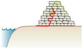
No matter how well you build a dike, extreme water pressure may cause water to seep through the dike or bubble up through the ground. It is advisable to have pumps with sufficient fuel and oil readily available to last the duration of the floodevent and an escape plan.
