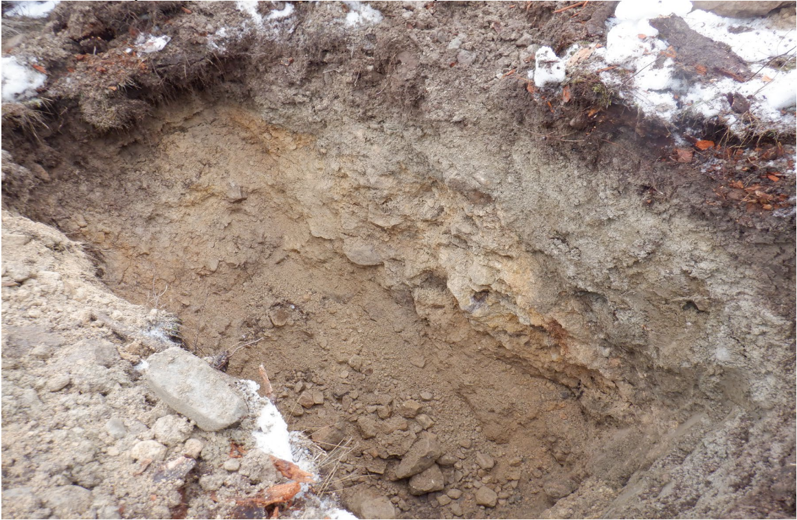
Photo #6 – testpit near upper station, 1.8m below grade.
