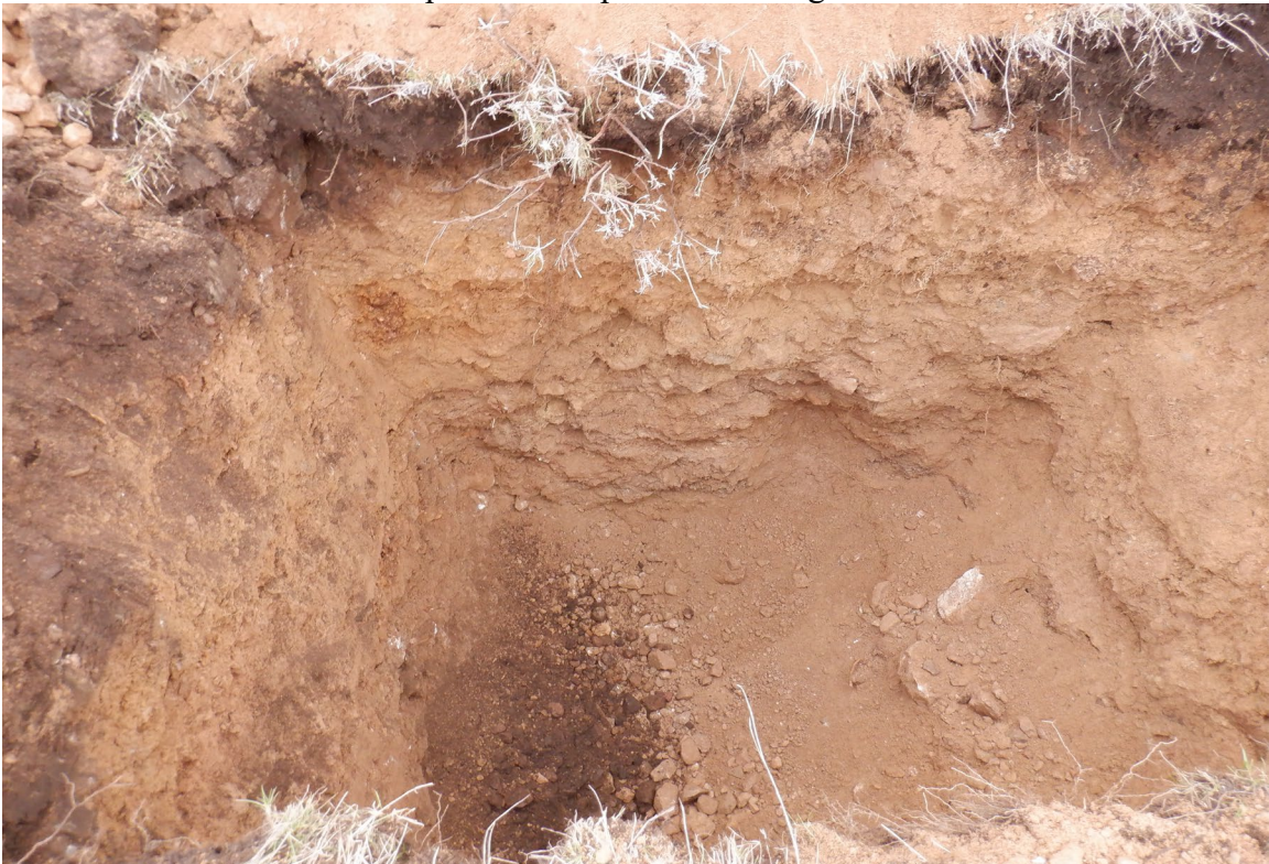
Photo #2 – bottom station testpit 2.0m deep with sand & gravel
