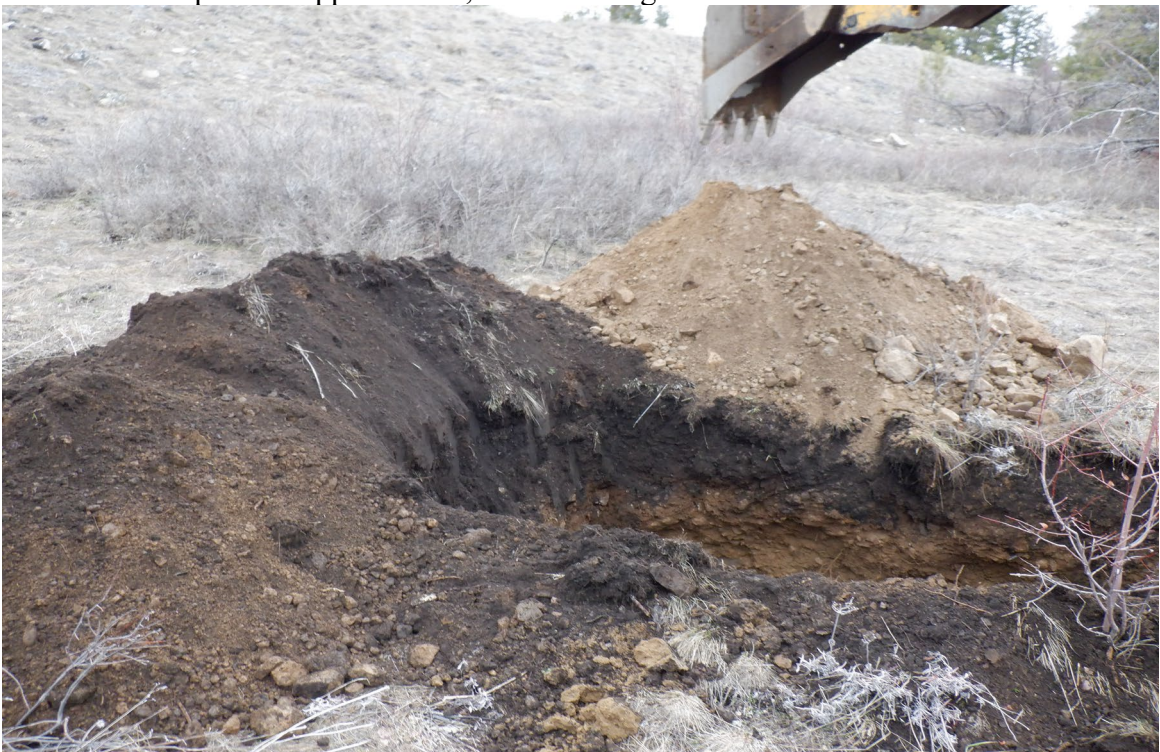
Photo #6 – testpit near upper station, 1.8m below grade.
