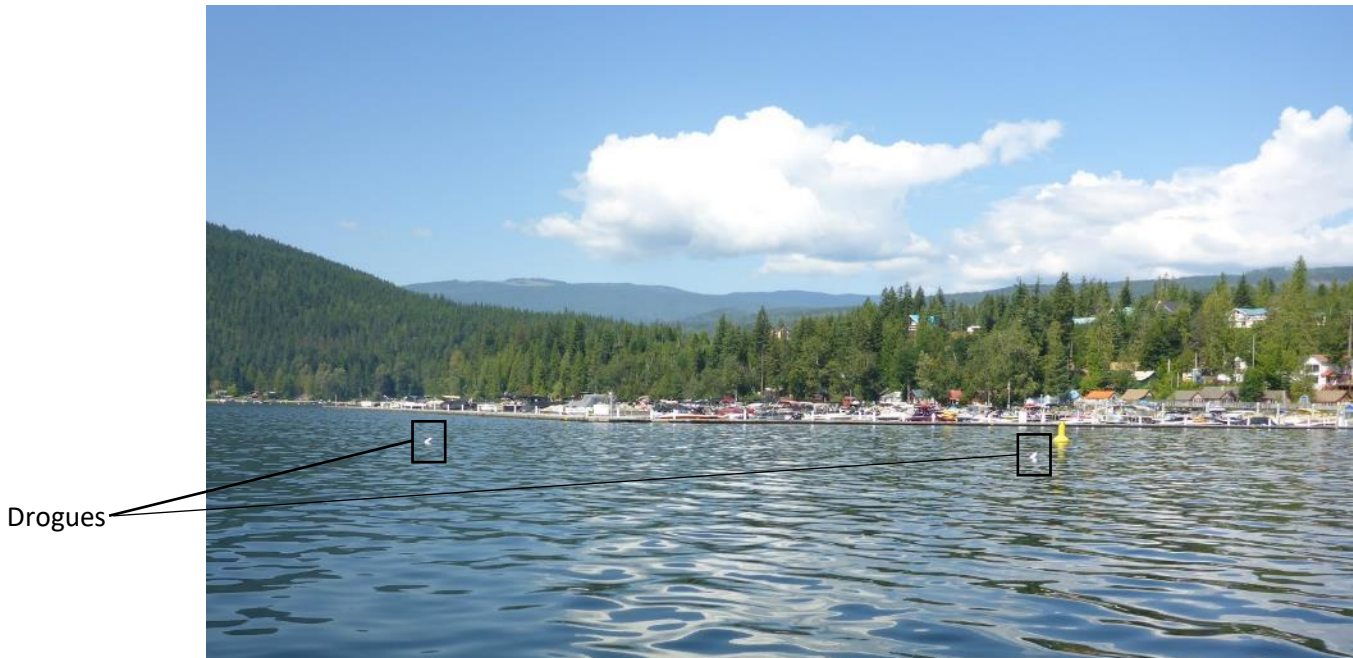
Figure 2: Photograph of drogue floats near current intake
