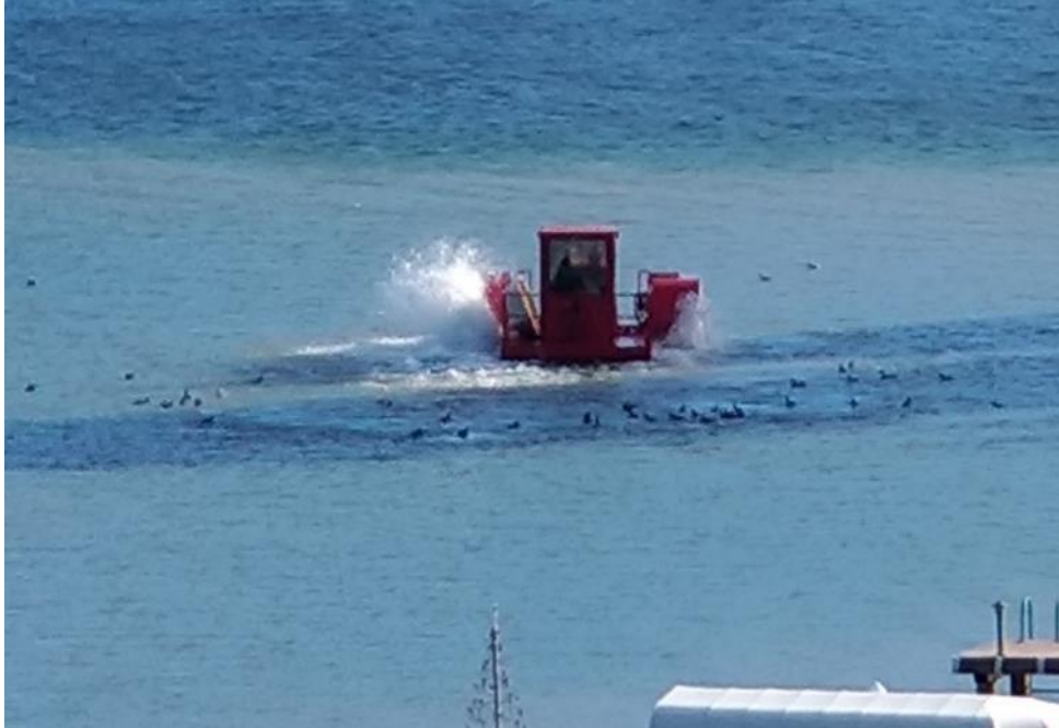
Figure A 1: Turbidity plume from milfoil rototilling machine
