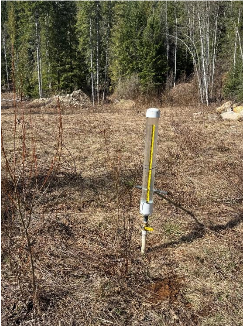
Photo 5: Lower bench permeability testing.
